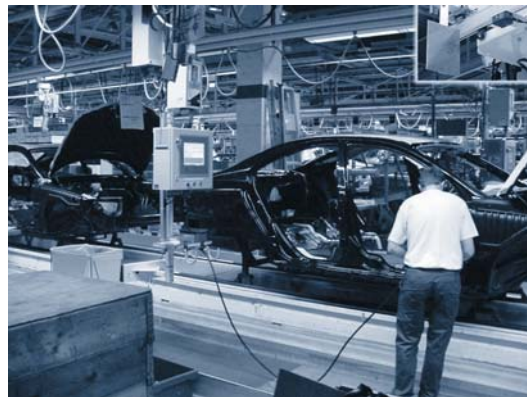
Operator shown using the electric screw driver which is being controlled by the CX1000 and Operator Interface
